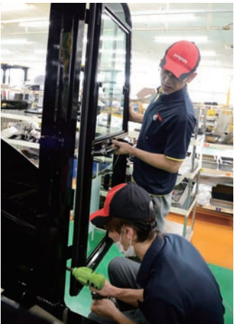
Bolt tightening work that used to be done by two persons can now be done by one
